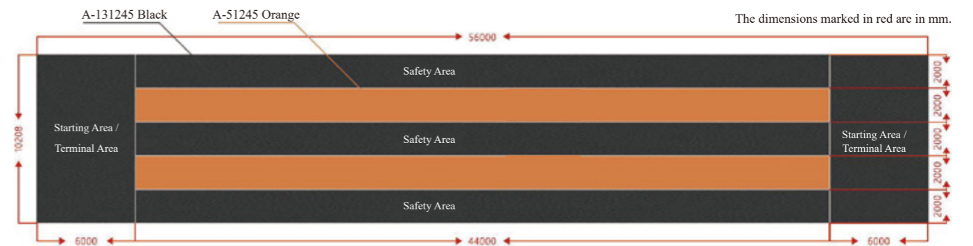
Parkour Track: Total length: 56m, width: 10.208m, track length: 44m, track width: 2m, safety zone length: 44m, width: 2m. Wide: 4.5cm
